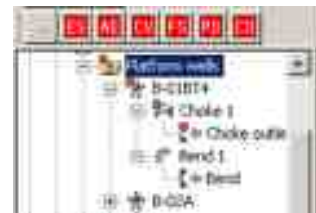
Figure 6.73: Expansion of the data tree to see which erosion node generates the alarm
