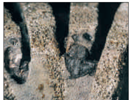
Balled Up (BU), Impregnated Bit
