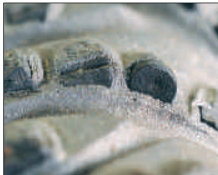
Worn Cutter (WT), Round TSP Broken Cutter (BT), Round TSP
