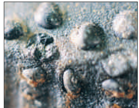
Broken Cutter (BT), Natural Diamond
