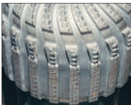
Ring Out (RO) on a TSP Bit
