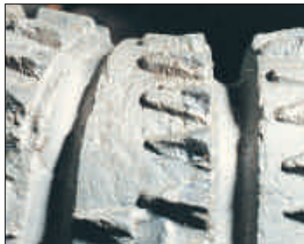
Worn Cutter (WT), Triangular TSP Broken Cutter (BT), Triangular TSP
