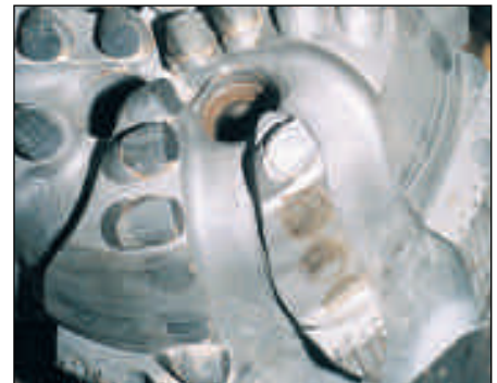
Ring Out (RO) on a PDC Bit
