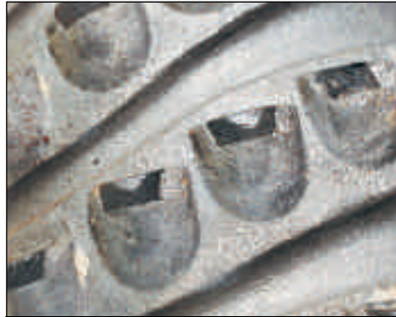
Worn Cutter (WT), Round TSP
