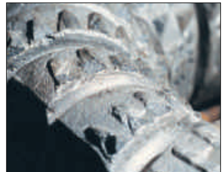
Broken Cutter (BT), Triangular TSP
