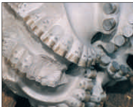
Junk Damage (JD), PDC Bit
